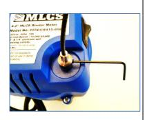
8. Find a suitable location to mount the remote variable speed knob and bracket. The knob and bracket can be removed (hex key provided) for installations that require through access (cabinets or dust enclosures).
