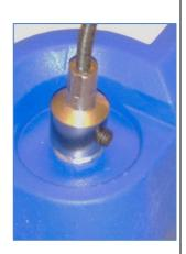
Tighten the coupler onto the variable speed accessory post.
