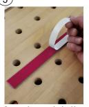
Remove the protective backing from replacement guide strip.
