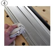
Using a shop cloth, remove excess glue residue with common adhesive removal product.
