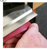
Clamp guide rail to work surface with Guide Strip hanging over edge. Apply strong downward pressure on corner of Guide Strip to break free.
