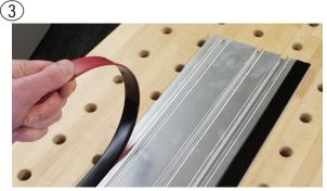
Flip guide rail over and remove guide strip. The guide strip is attached with strong adhesive but is able to be removed.
